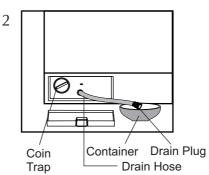
Place a shallow container near the bottom door. Pull out the drain hose and open the drain plug to drain out the water from the machine in the container.
